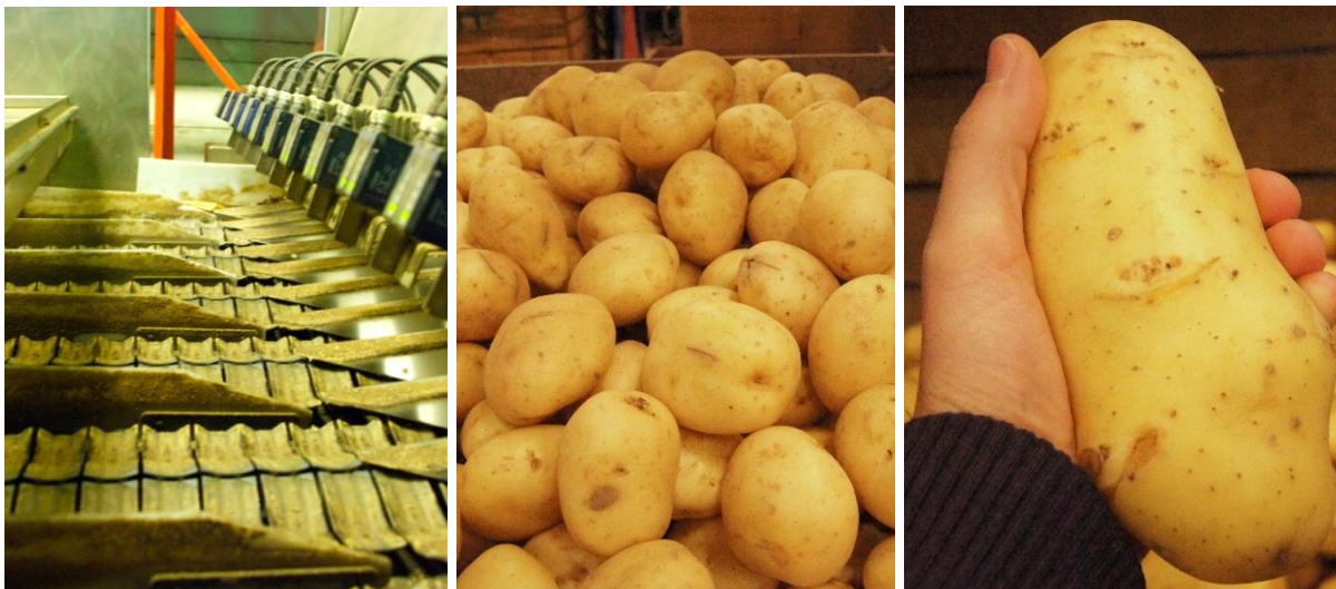
Optical sensors are used to detect surface defects in potatoes. Potatoes of a size within 42 to 65 mm and acceptable visual quality are sold as fresh food potatoes. Potatoes of other sizes are sold to the food processing industry. Hvebergsmoen Potetpakkeri AS, June 2013. (Photo: Bioforsk S. Adler, SINTEF E. Bar)
