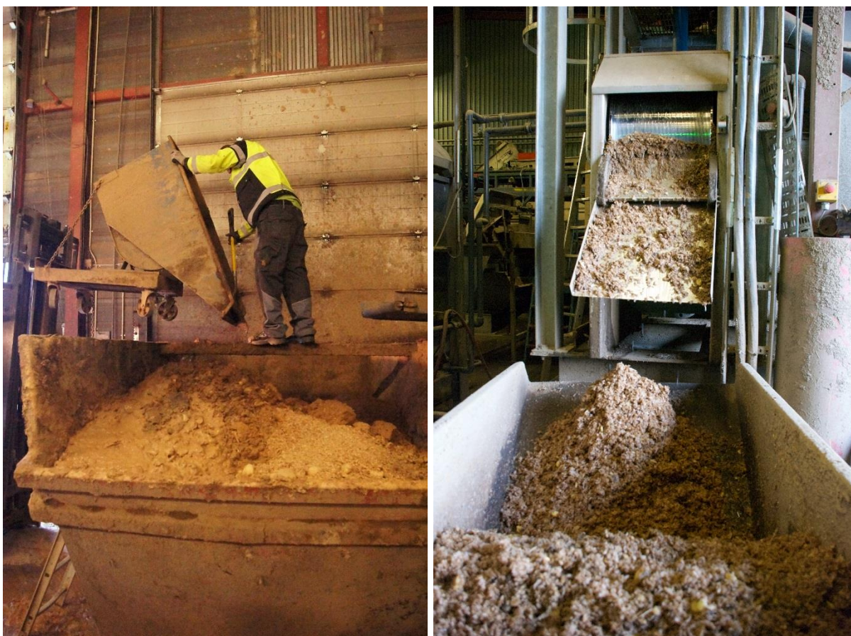
Potato residual soil with organic material (left). Separation of organic material from process water allows recycling of water (right) at Hvebergsmoen Potetpakkeri AS, and significantly reduces the water consumption, June 2013. (Photos: SINTEF E. Bar, Bioforsk S. Adler)
