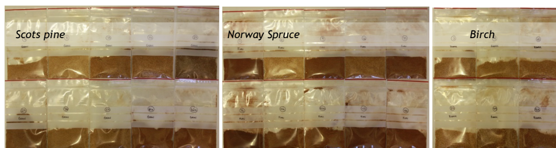
Figure 3.3. Dried and homogenized bark samples of Scots pine, Norway spruce and Downey birch.
