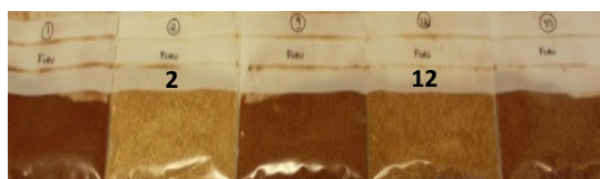
Figure 3.6. A higher content of inner bark gave the bark from 40 year old pine (no. 2 and 12) a more yellow appearance, as compared to the brown, predominantly outer bark from the older trees.
