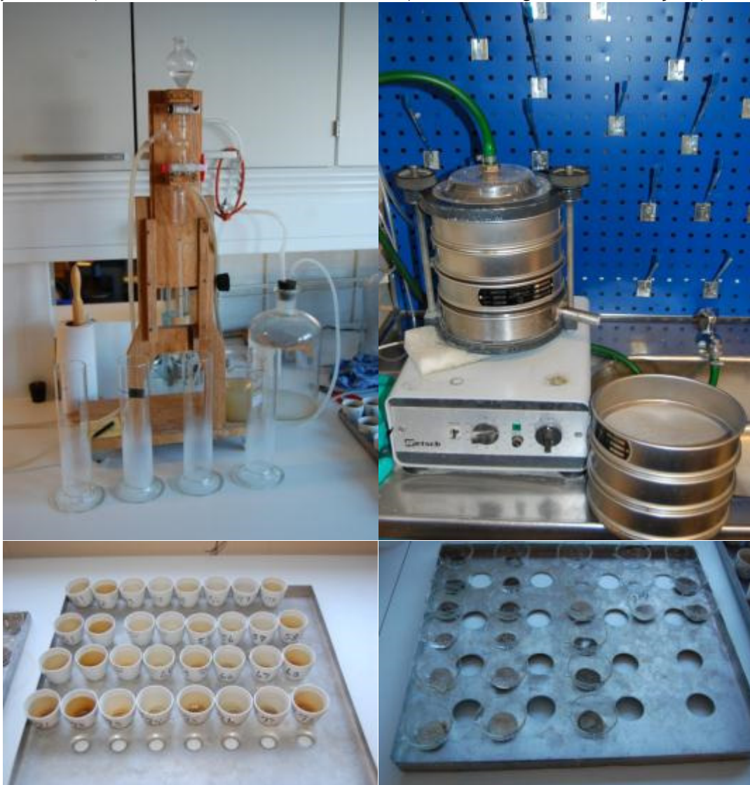
Figure 4.4. Equipment used for mechanical analysis. Left: Setup for pipetting of silt and clay sedimentation samples. Right: Wet sieve shaker used for separating sand fractions (Retsch).
