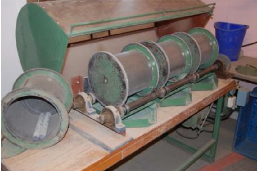
Figure 4.2. Rotating 2 mm sieves used for separating gravel from fine earth (constructed at Kise Research Station).
