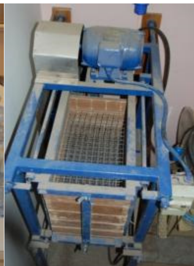
Figure 4.7. Sieve shaker for aggregate separation (Kise).
