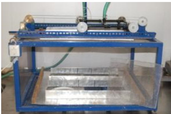
Figure 4.8. Rain simulator used for measuring soil aggregate stability (Kise Res. Stn.).
