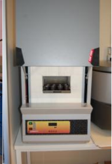
Figure 4.3. Furnace used for ignition-loss analysis (Carbonite).
