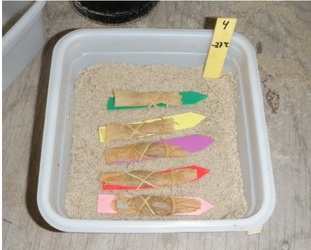
Photo 9. Tiller groups in plastic tray filled with moist sand. The tiller groups were completely covered with sand before transfer to the freezing chamber. Photo: Trond O. Pettersen.
