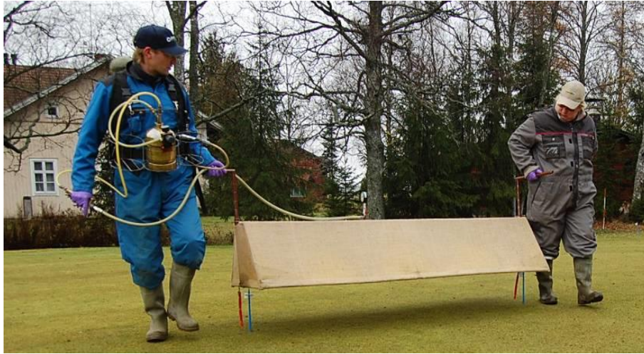
Photo 3. "van der Weij" -type plot sprayer used in trials at Loimijoki. Photo: Oiva Niemelainen.
