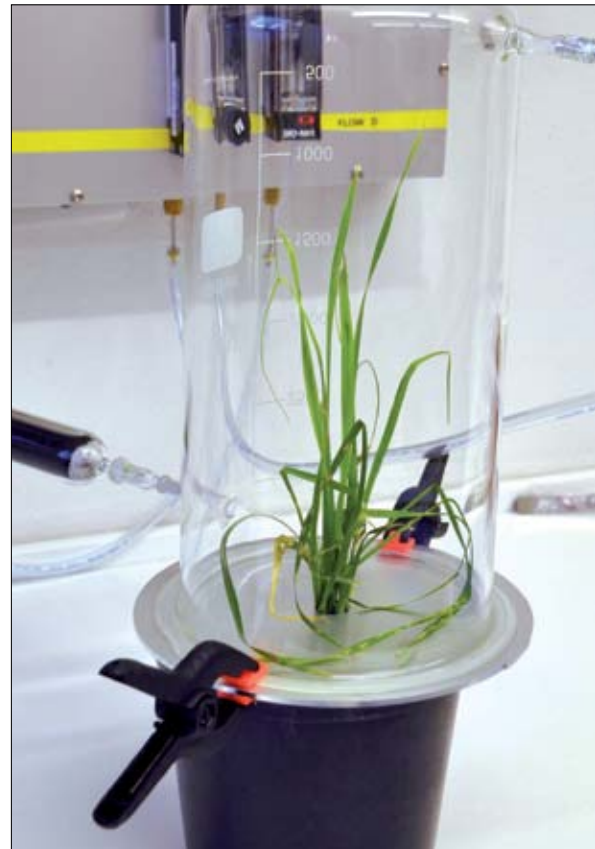
Figure 4. VOC collection of wheat plants inoculated with B. graminis in glass chamber. Photo: A. Ficke.
