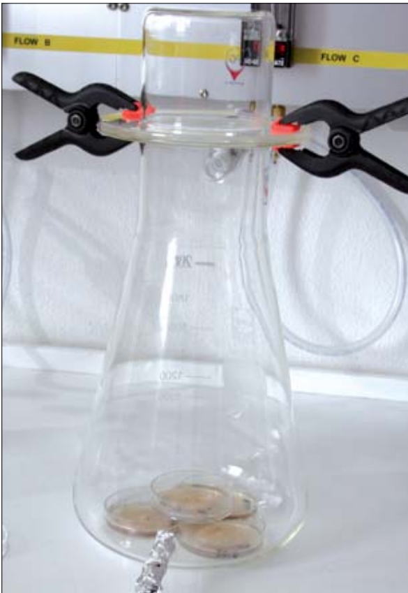
Figure 3. VOC collection of S. nodurum cultures in glass chambers. Photo: A. Ficke.
