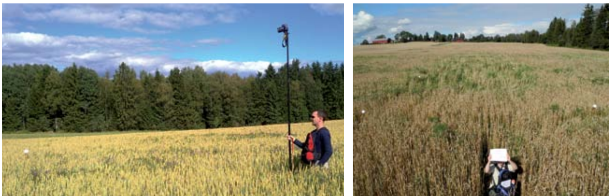
Figure 1. Left image: Camera set-up. Photo: T.W.Berge. Right image: Captured perspective view image (plot no. 5, field 1) at harvest time (September 1st). White balls delimit the 8.0 × 8.0 m plot. Photo: Steve Goldberg.
