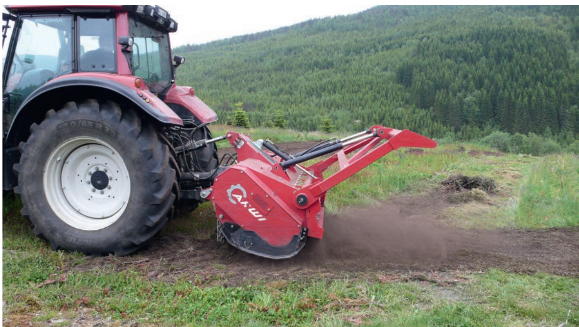
Figure 1. Grinding of stumps before planting a new generation of Christmas trees. Norway 2012. Photo: V. Talgø
