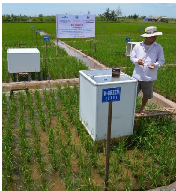
Figure 4. Field trials in Nam Dinh province to measure \text{CH}_4 and \text{N}_2\text{O} emissions from rice grown under three nitrogen regimes.
