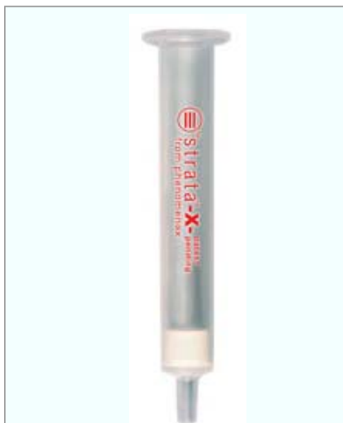
Figure 7. SPE-cartridge with a Phenomenex Strata-X sorbent.
