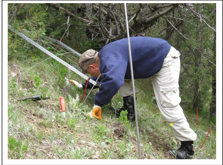
Fig. 3.1. Measuring inclination of a 1-m 2 plot at the Gauyan monitoring site.
