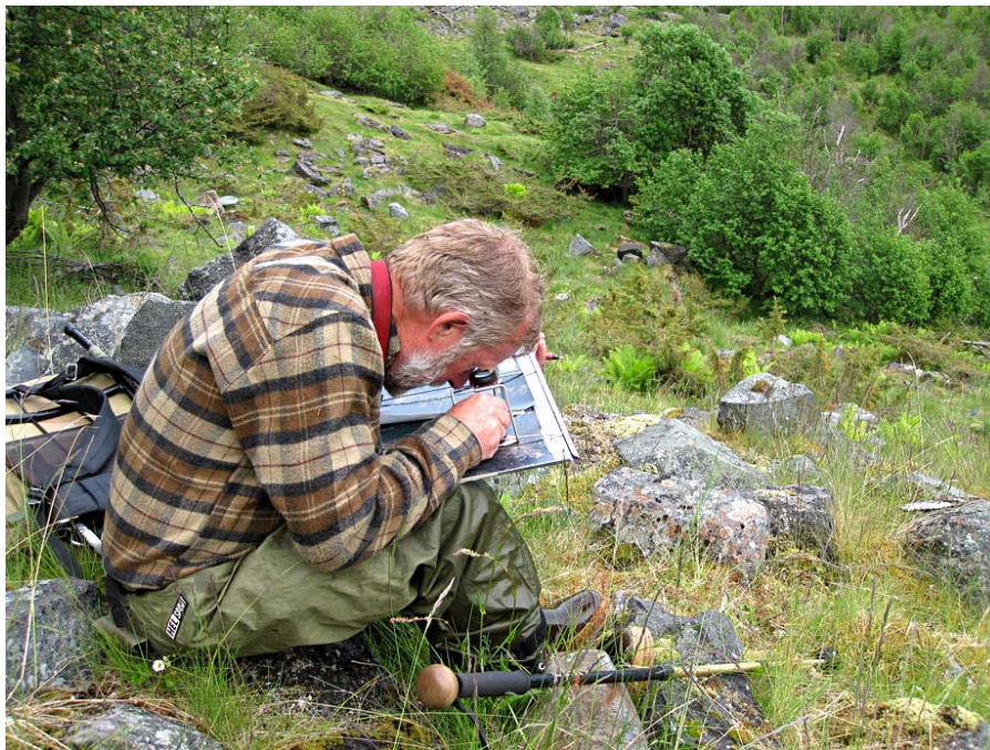
Figur 10. Per Bjørklund drawing a land cover map on a stereo pair of aerial photographs during work in 2009. Photo: Linda Aune-Lundberg, Skog og landskap.
