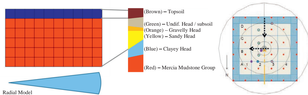
Figure 3 (left) Schematic illustration of the vertical extent of the ASgard plot models. Note that in the version of the model used here, the soil/rooting zone may be multiple compartments deep and the compartment sizes are radially uniform on a log-scale. (right) Plan view of radial grid (up to the edge of the rooting zone) overlaid on diagram of experimental sampling quadrants
