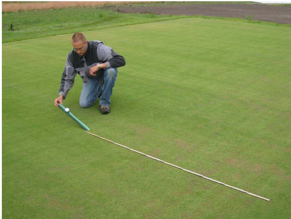
Photo 3. Research technician Trond Pettersen measuring ball roll distance using a modified stimpmeter with 38 cm distance from the notch to the beveled end. Photo: Trygve S. Aamlid.
