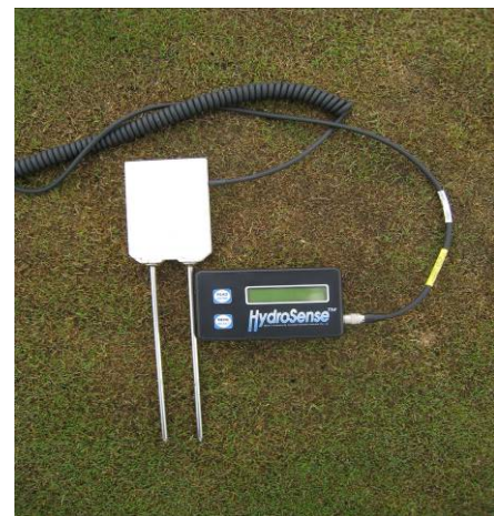
Photo 6. TDR instrument with 20 cm probe used for measurement of volumetric soil water content. Photo: Trygve S. Aamlid.
