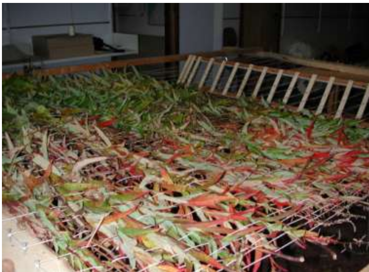
Figure 6. Small-scale hand-made production of erosion control mats based on fireweed. Photo: Hermod Nilsen.
