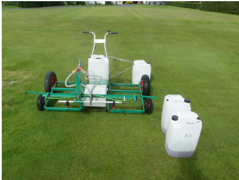
Photo 2. Experimental sprayer used for liquid fertilizer applications.
