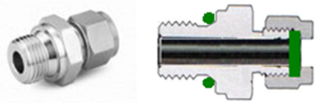
Fig. 6 Sampling port, made from a standard Swagelok male tube fitting, where the locking cones were replaced by a GR-2 septa
