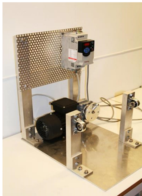
Fig. 10 Photobioreactor stand, including motor, rotating disc, transmission, frequency converter, and holders for the culture vessel
