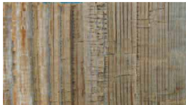
Fig. 11. Characteristic rot caused by C. borealis with small cubes and white mycelium. Photo: H. Solheim
