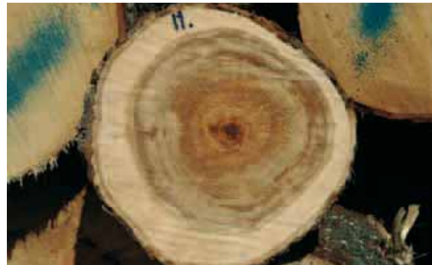
Fig. 10. End of a log (no. 11 at Kittelbu) with C. borealis rot. Note the zone surrounding the rot. Photo: H. Solheim
