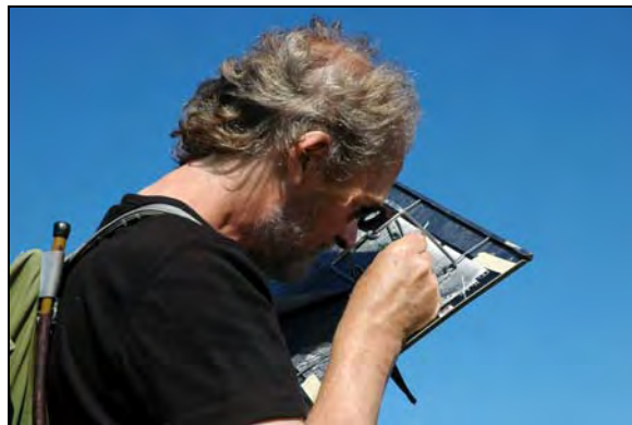
Figure 4: Yngve Rekdal shown drawing a land cover map on a stereo pair of aerial photographs during field work in 2005. Photo: Geir-H Strand © NIJOS.
