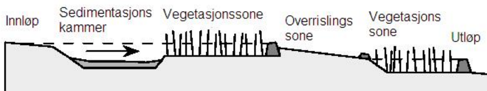
Figur 2: Prinsippkisse for en fangdam.
