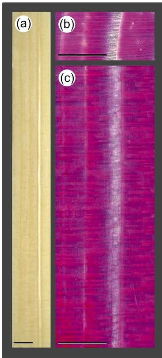
Fig. 2. Phloxine B staining experiment of a lucid band (LB) in Norway spruce sapwood (annual ring 2006) from Ekebo (southern Sweden). In the never dried and fully saturated state, the LB regions have a lighter, almost white, colour compared to the surrounding wood (a); LB remain unstained when flow experiments with the Phloxine B solution are performed. The transverse view is shown in (b), the radial longitudinal view in (a) and (c), reference bars=3 mm.
