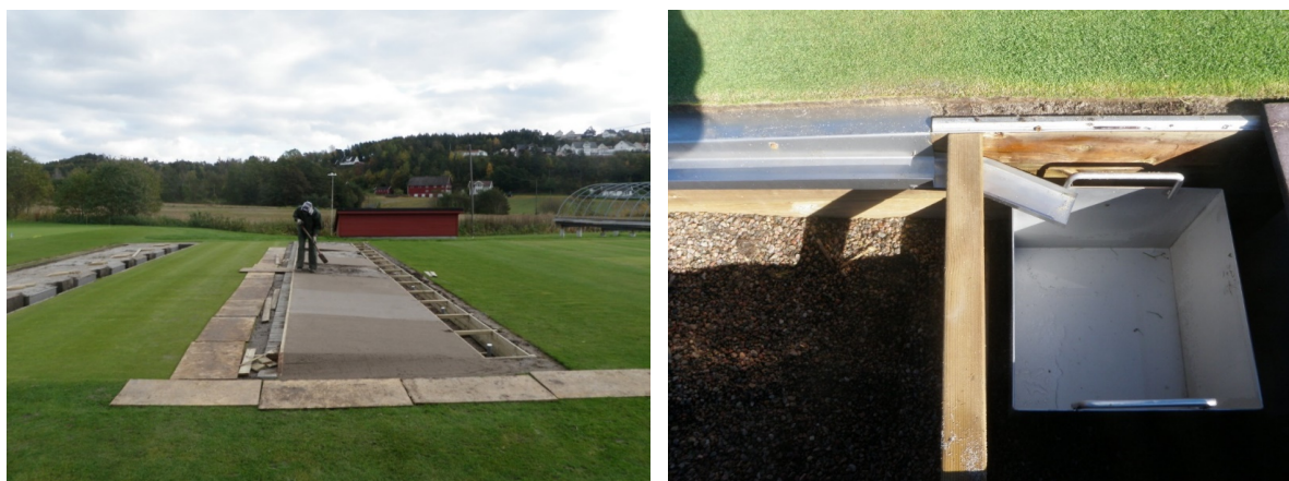
Photo 2 a,b. Remodeling of lysimeters in 2015 to allow for collection of surface water. Photos: Trygve S. Aamlid
