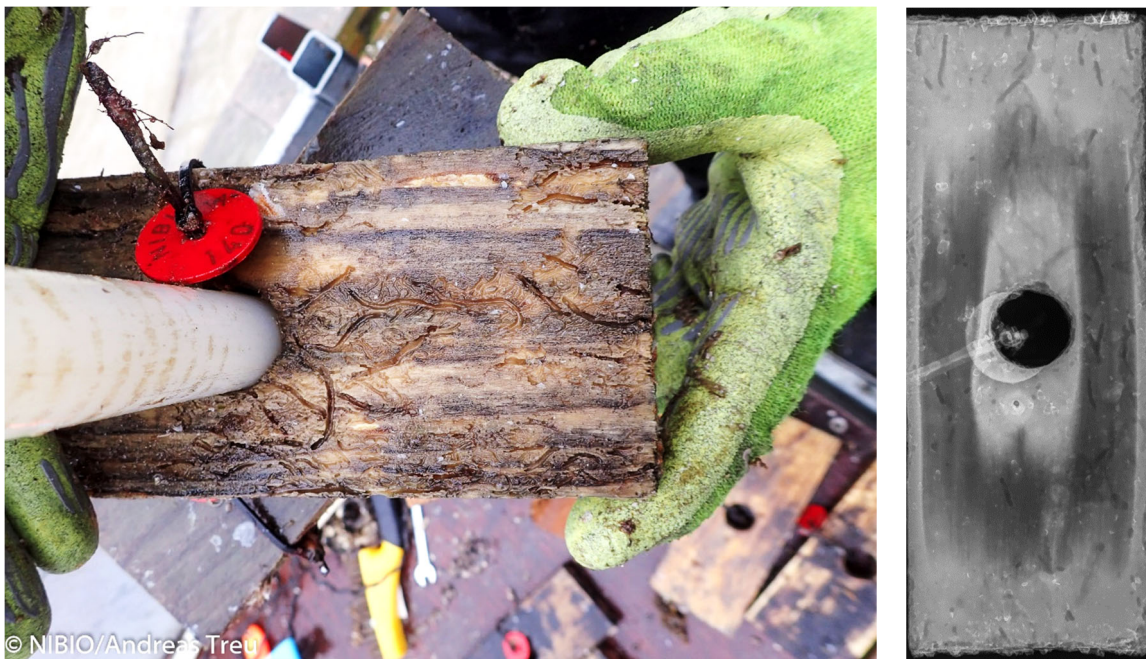
Figure 9. Gribble attack on spruce wood samples at the test site in Drøbak; tunnels are even visible in the x-ray image (right)
