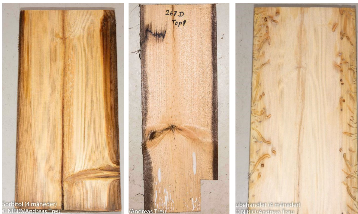
Figure 14. Radial section of treated wood poles; satric (left), creosote (middle) and untreated (right)
