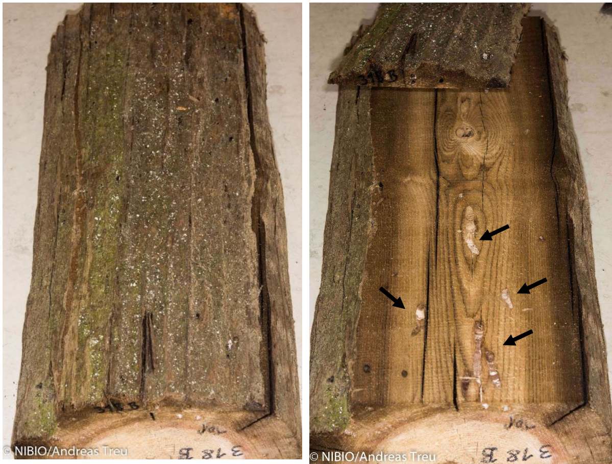
Figure 2. Suberficial degradation of creosote treated wood pole (left) and borer attack (right). The 9 m long pole was removed from Hesselbergbrygga/Moss
