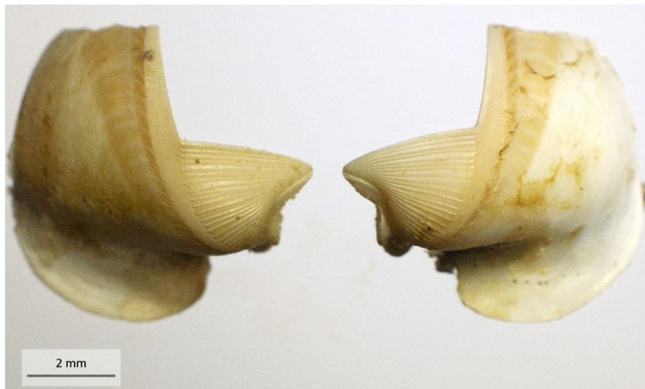
Figure 8. Shell valves from shipworm found in the heartwood zone of creosote treated Scots pine poles exposed in Moss harbour, the extending shell auricles could point to the species Psiloteredo megotara
