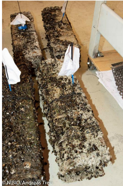
Figure 16. Wooden steps after 4 month in the Oslofjord
