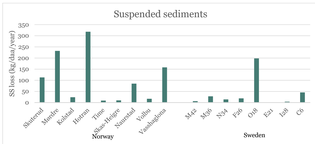
Figure 4.4: Average suspended sediment losses in Norwegian and Swedish catchments (Bechmann et al. 2017; Kyllmar, pers. comm.).
