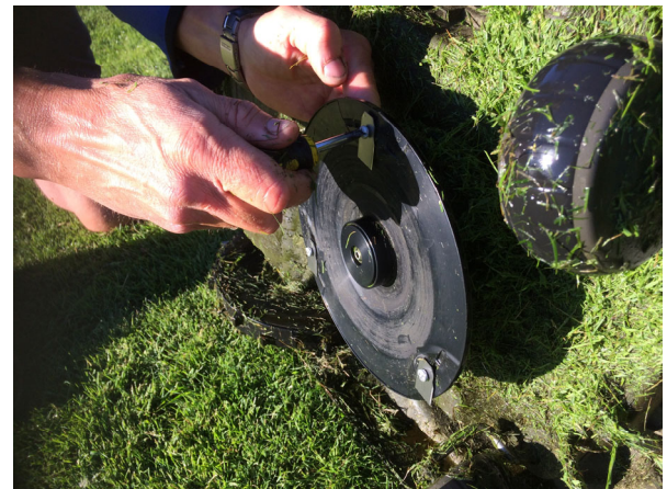
Photo 6. First replacement of knives on robotic mowers, 25 Aug. 2020. The knives on fairway mowers (top left) had more signs of wear than the knives on semi-rough mowers (bottom left). Photos: Anne F. Borchert.
