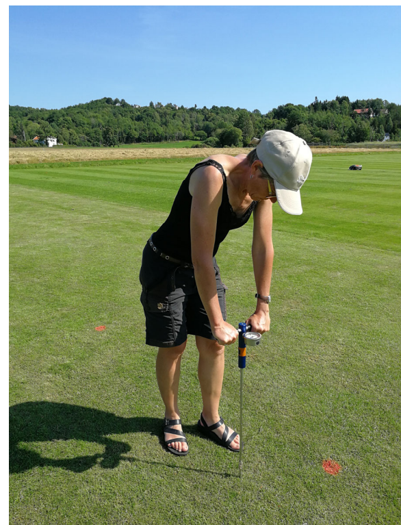
Photo 9. Karin Juul Hesselsoe measuring start values for soil penetrometer resistance on 12 Aug. 2020. Photo: Anne F. Borchert.
