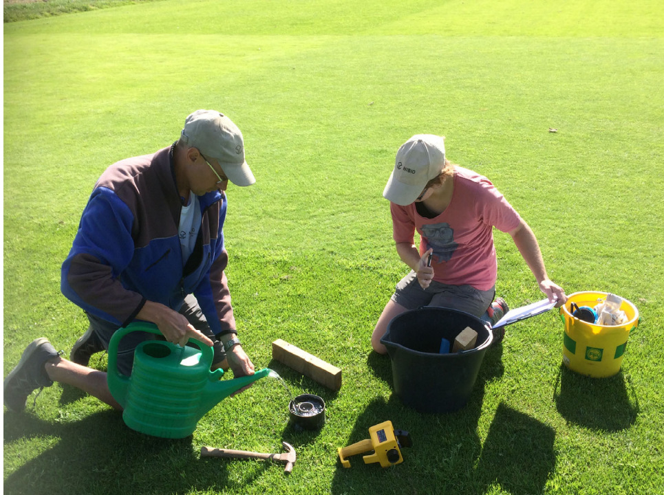
Photo 10. Infiltration measurements on 4 Sep. 2020. Photo: Trygve S. Aamlid
