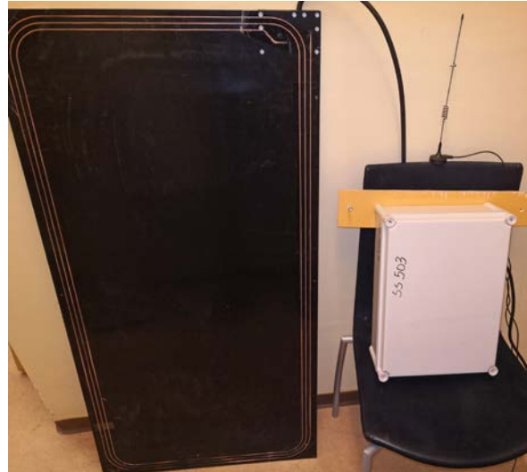
Orru sáddejeaddji/registrerenrusttet (olgeš bealde) mas lea pláhttaanteanna, maid Biocontrol AS fitnodat lea ráhkadan. (Govven: Erlend Winje).
