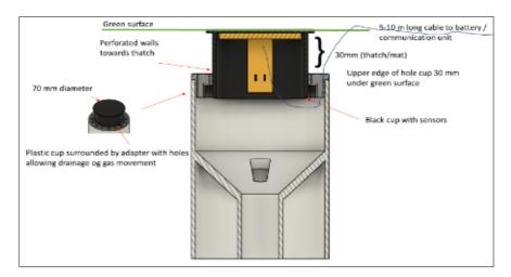
Figure 2. Sensors embedded in a black cup were mounted in a hole cup via a perforated adapter.
