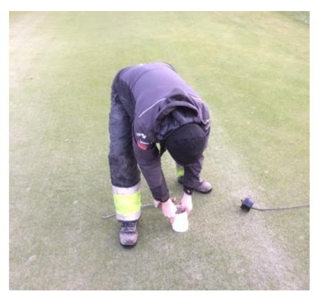
*Photo 2. The sensors were fitted into a hole cup. Top of hole cup was 3 cm from green surface, thus not inhibiting gases from the thatch layer to penetrate to the sensors. Photo: Trygve S. Aamlid*
