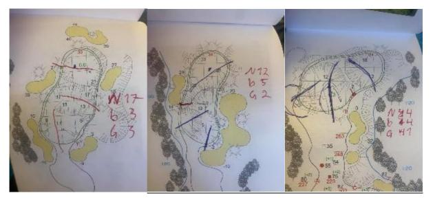
Figure 23. Examples of the simple, unbranched ventilation systems laid out under the covers at Holtsmark GC. N=green nr, b=treatment, G=block. Drawings: Mads Thers.
