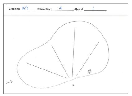
Figure 4. Sketch of drainage pipes installed on green 'Blue 9' at Haga GC. Placement of blower for ventilation (x) and hole cup with sensors (s) are indicated. Drawing: Gavin Jagger.
