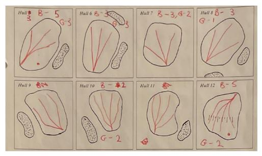
Figure 16. Ventilation systems on some of the greens at Asker GC. (B=Treatment, G=Block (replicate)). Red dots on greens indicate sensor placement. Drawing: James Bentley.
