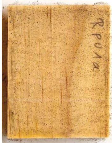
Figure 10: Surface of untreated and furfurylated Radiata pine after 5 and 11 weeks of exposure to a surface fungi mix
