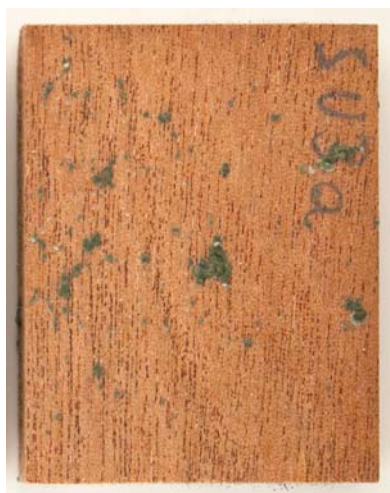
Figure 13: Surface of untreated sipo mahogany after 5 and 11 weeks of exposure to a surface fungi mix
