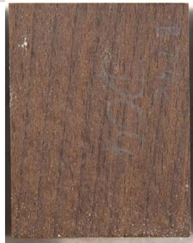
Figure 12: Surface of untreated and furfurylated beech after 5 and 11 weeks of exposure to a surface fungi mix
