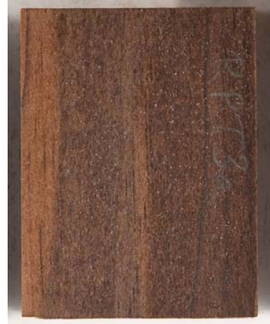
Figure 10: Surface of untreated and furfurylated Radiata pine after 5 and 11 weeks of exposure to a surface fungi mix
