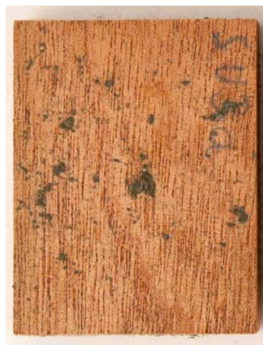
Figure 13: Surface of untreated sipo mahogany after 5 and 11 weeks of exposure to a surface fungi mix
