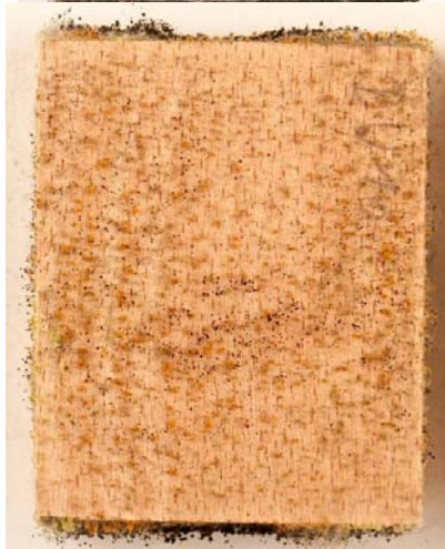
Figure 12: Surface of untreated and furfurylated beech after 5 and 11 weeks of exposure to a surface fungi mix
