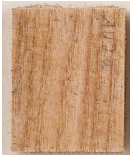
Figure 11: Surface of untreated and furfurylated ash after 5 and 11 weeks of exposure to a surface fungi mix
