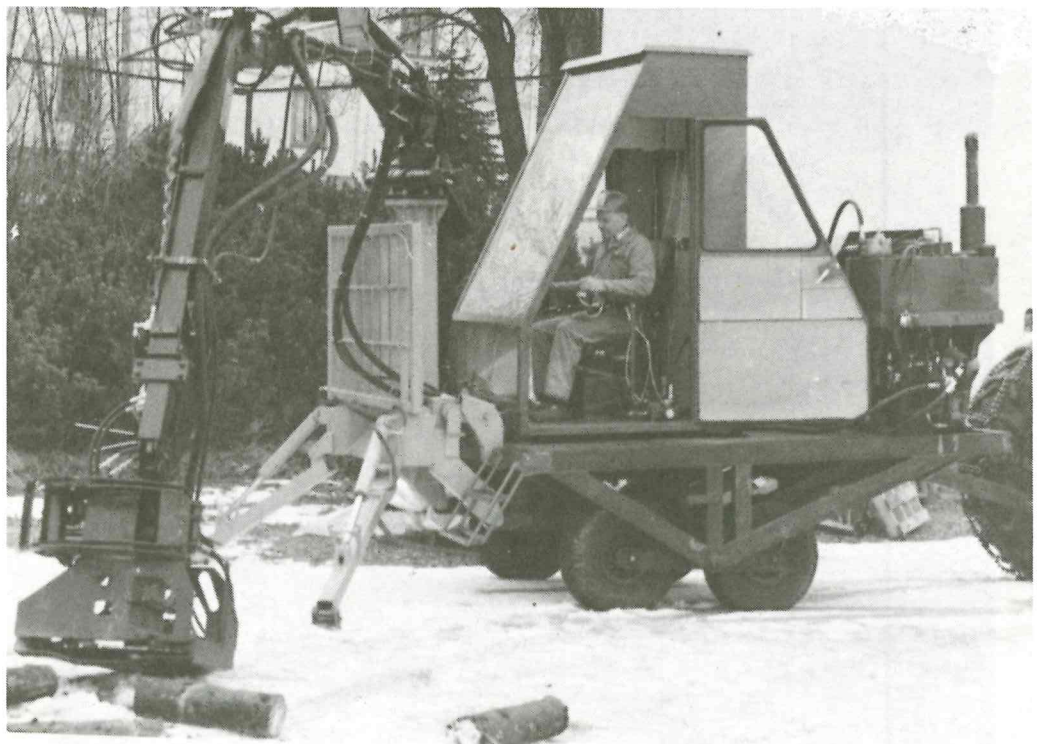
Fig. 26. The trailer-mounted test machine for measuring performance differences, may be transported after a tractor or a truck to the research area.
