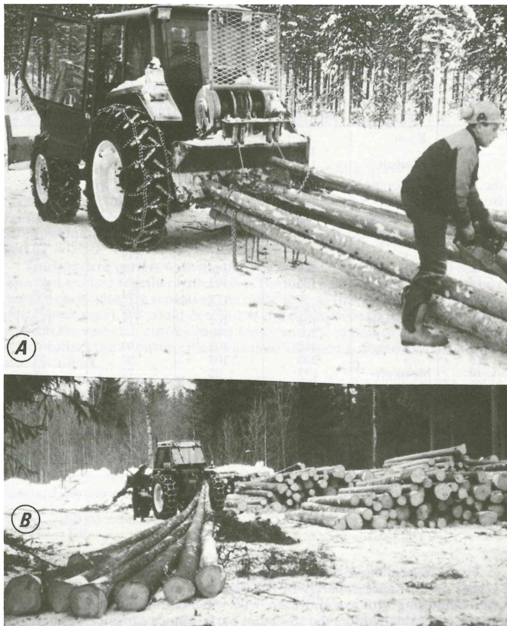
Fig. 24. «Ground» skidding of stems by agricultural tractor. Time studies of tractor transport. A: Terminal operation. B: Underways operation (GJEDTJERNET 1989)
