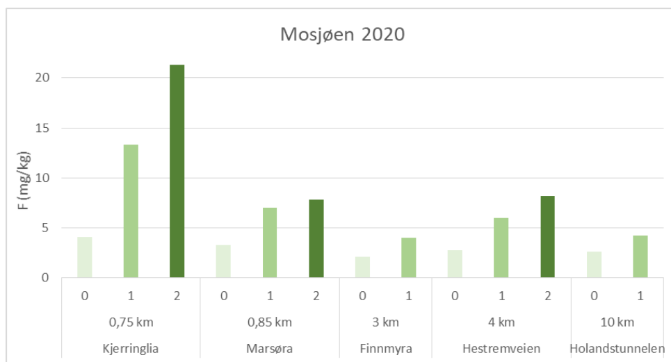
Figure 3.6. Mean F-concentrations in pine needles of different ages at Hydro Årdal (upper panel), Hydro Sunndal (middle panel) and Alcoa Mosjøen (lower panel) smelters, sampled at different distances from smelters during 2020. Pine needles "0" are current-year needles, "1" are one-year-old needles and "2" are two-year-old needles.
