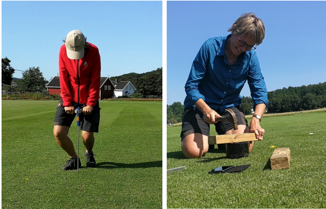
Photo 9: Soil compaction (left) was measured in August on both fairway and semi-rough. A double ring infiltrometer (right) was knocked into the turfgrass surface before filling with water to measure infiltration rate.
