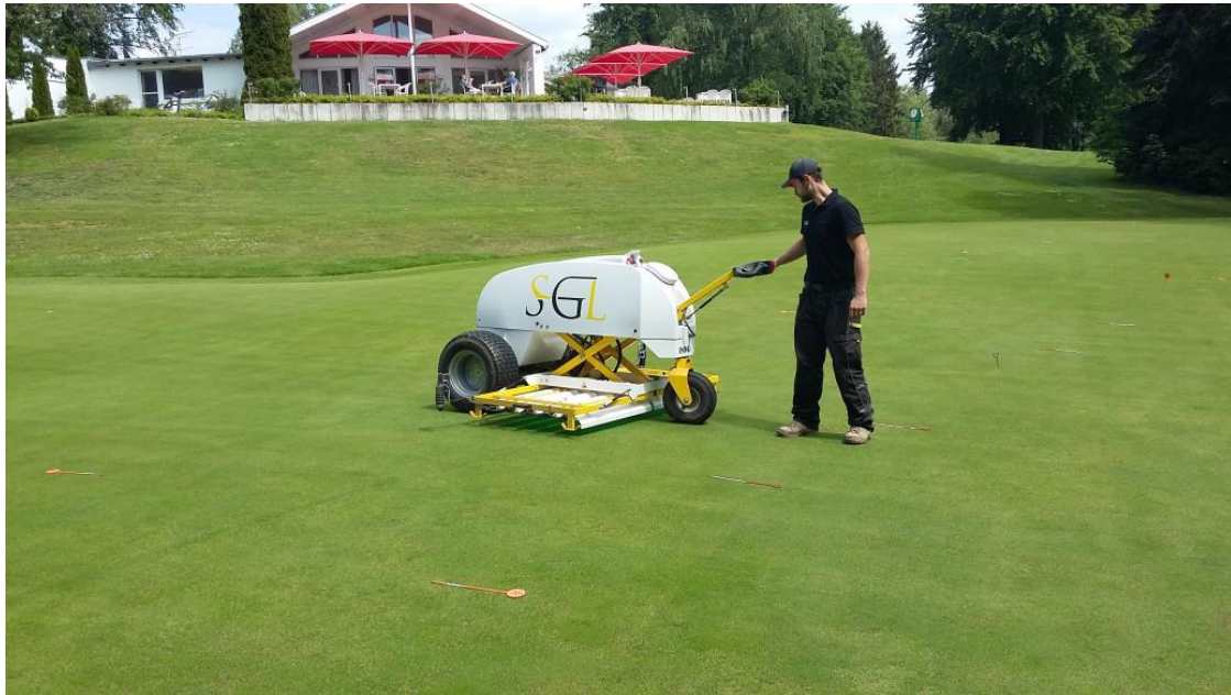
Photo 10: SGL UVC 180 radiation unit operating on experimental green.
