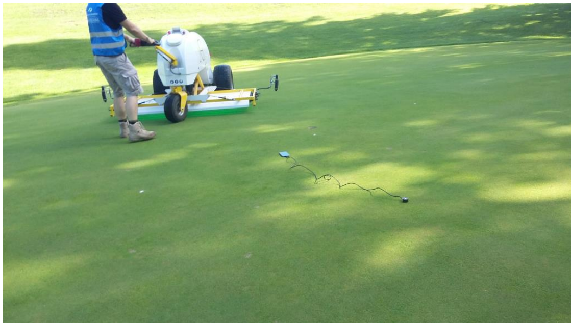
Photo 11: SGL UVC 180 unit operating on trial plot, dosage controlled by device.
