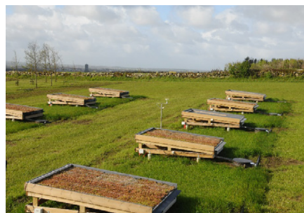
Figure 3. Experimental roof on NIBIO Særheim where different compositions of substrate and vegetation are examined. Photo: Arne Sæbø
