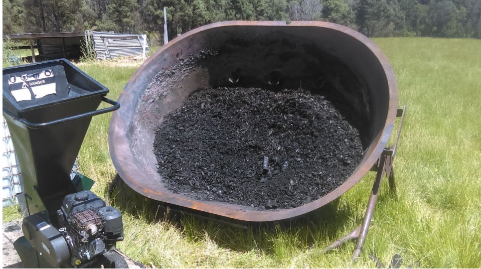
Fig. 6.4. 1850 Liter Kontiki Stretch kiln from Terra preta Developments in Tasmania Australia. Biochar is grinded to a finer particle size using a 6 hp garden shredder. Photo: www.terrapretadevelopments.com.au
