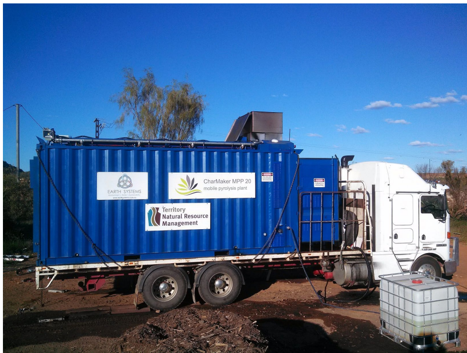
Fig. 6.5. Charmaker MPP from Earth Systems Pty Ltd (Australia) Photo: esenergy.com.au
