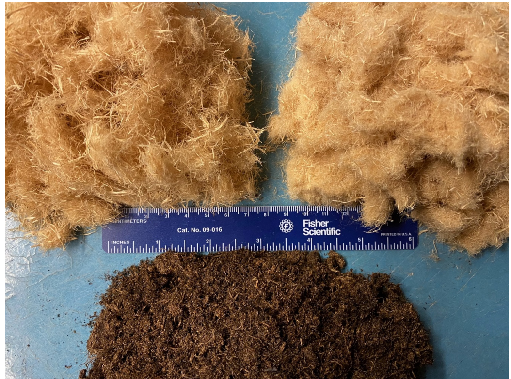
Figure 1. Coarse (top left), fine (top right) Picea abies engineered wood fiber, and H2-H4 sphagnum peat moss (bottom) tested in these experiments.
