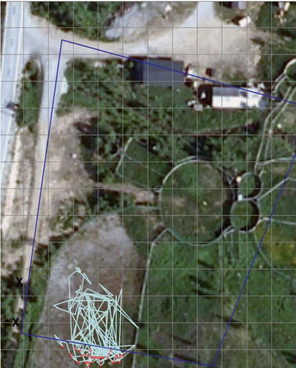
Physical fencing system and virtual fenceline (blue line) set by GPS endpoints in each corner. The line which animals could cross was just within the lower end of their experimental enclosure.
