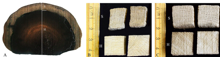
Fig. 1 Cross section of the archaeological waterlogged oak log with two clearly visible wood layers: sapwood (S) and heartwood (H) (a), exemplary air-dried untreated (b) and MTMS-treated (c) waterlogged samples
