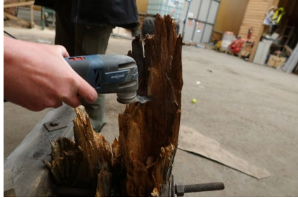
Cable car trestle 87889-16, object 2. Cutting of sample 2A8
