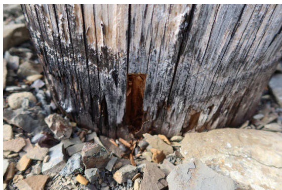
Leg NW, soil contact, after sampling
