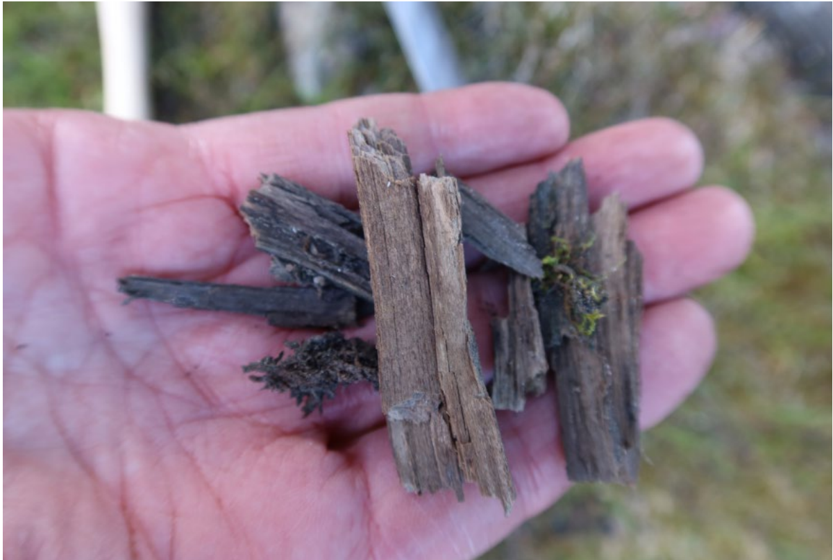
"Taubanestasjonen", 93041-14. East side. Sample taken from wood in ground contact, directly below the point of drilling
