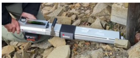
Resistance drill (IML-RESI PowerDrill PD400)
