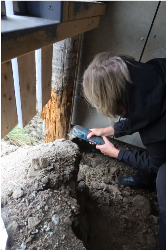
Hotel Radisson Blu, foundation pile SAS1. Cutting sample SAS1-2, 60 cm from beam
