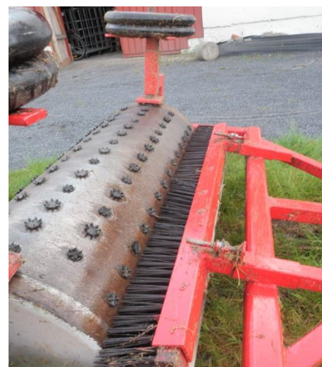
Photo 2. Friction wear drum used in trial in 2012. Photo: Trygve S. Aamlid
