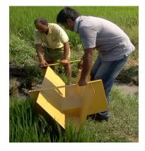
Measuring irrigation water through RBC flume:
