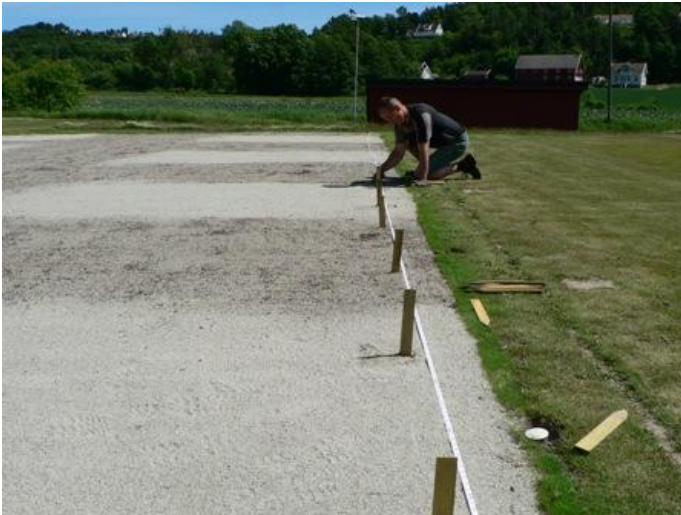
Photo 1. Research technician Atle Beisland prepares lysimeter plots trial for sowing, 22 June, 2010. Note that Green Mix rootzones had a darker colour than straight sand rootzones. Photo: G. Kusliene.
