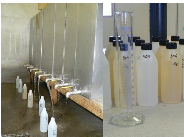
Photo 6. Leakage water was collected for N and P analyses. Photo: G. Kusliene.
