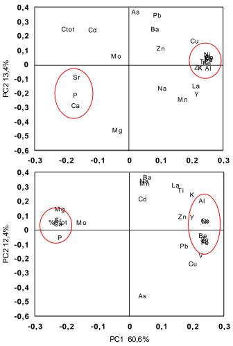
Fig. 5.5. Parameter loading along the two first principal components in a PCA analysis of soil data from the A horizon (top graph) and B horizon (bottom graph), explaining 69.1 and 73.0% of the variation in soil elemental composition, respectively.
