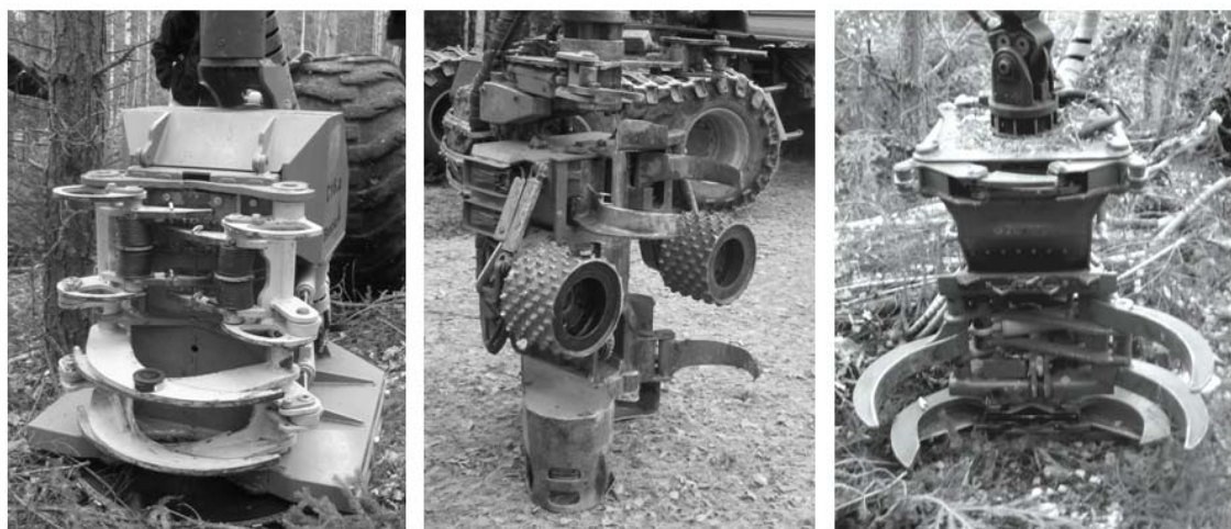
Figure 1; The heads used in the study. From the left; Bracke C16a, Log Max 4000B, and Naarva-Grip 1500-40E.
