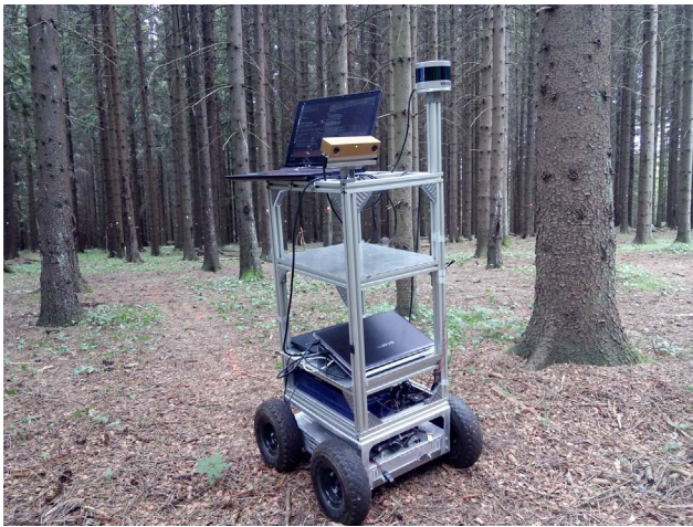
Fig. 3. The mobile platform used for data collection purposes, based on the 'Superdroid 4WD IG52 DB' rover. The grey and black cylinder at top right is the VLP-16 LiDAR. The golden rectangular device at top left is the Bumblebee stereo vision camera.
