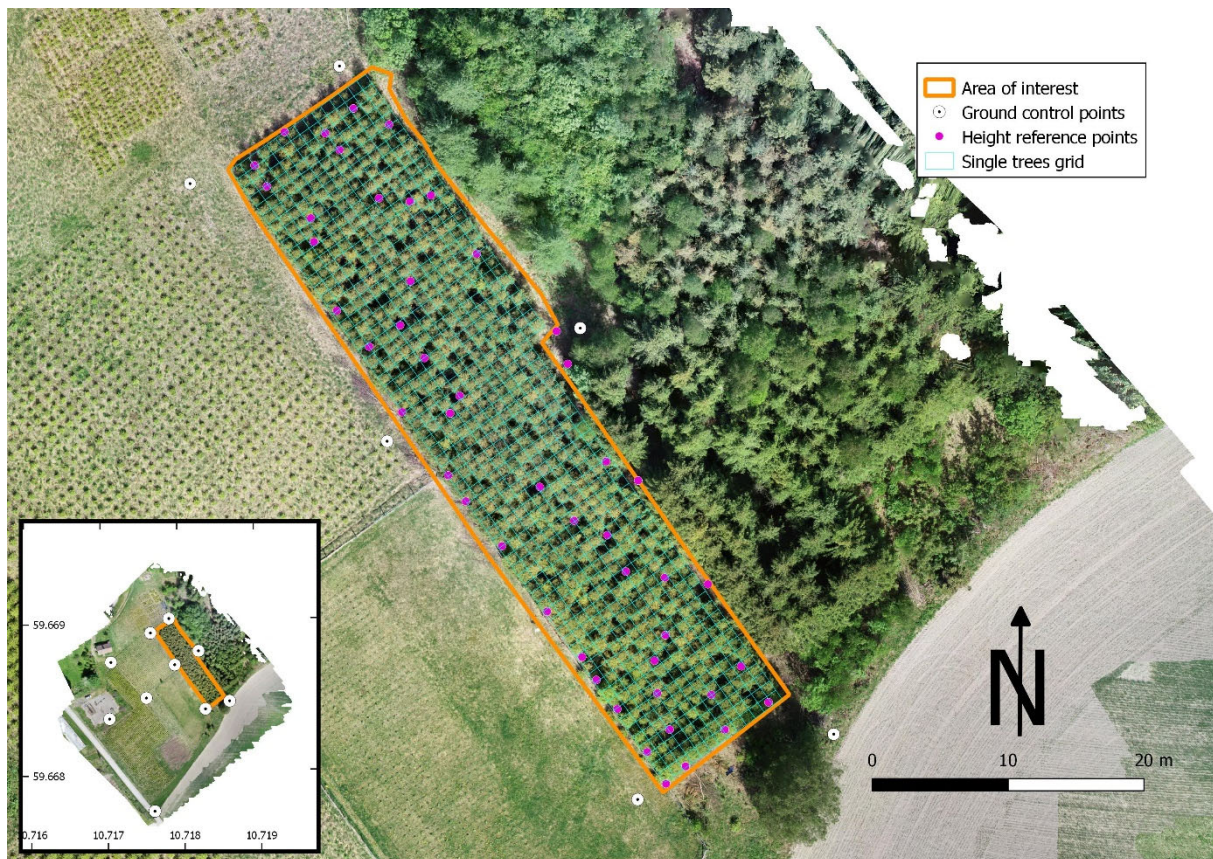
Figure 1. Overview of the study area including the locations of the ground control points, height reference points and the single tree grid cells.
