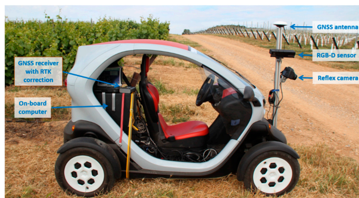
Figure 2. Electric platform equipped with an on-board computer for autonomous navigation and signal processing. The Kinect v2 sensor was installed on an adjustable height structure, provides RGB and distance information associated to Global Positioning System (GPS) coordinates.
