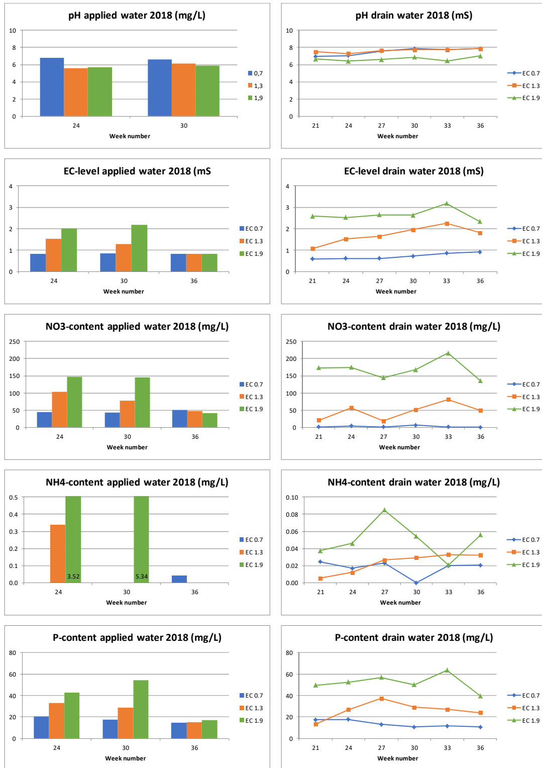
Figure A3.1. Course of pH, EC and levels of nutrient elements in applied drip and drain water of 'Discovery' trees grown at three levels of EC- fertiligation in pots in a greenhouse at NIBIO-Særheim in 2018.
