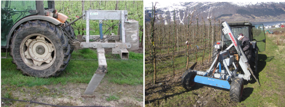
Figure 9. Root pruning devices with vertical knife (left) and hydraulic slant knife (right) mounted on back side of tractor (photos: F. Maas and M. Meland).
