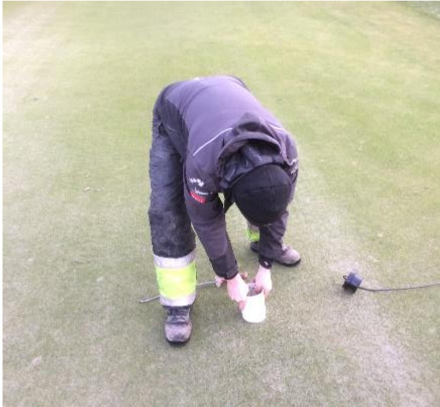
*Photo 2. The sensors were fitted into a hole cup. Top of hole cup was 3 cm from green surface, thus not inhibiting gases from the thatch layer to penetrate to the sensors. Photo: Trygve S. Aamlid*
