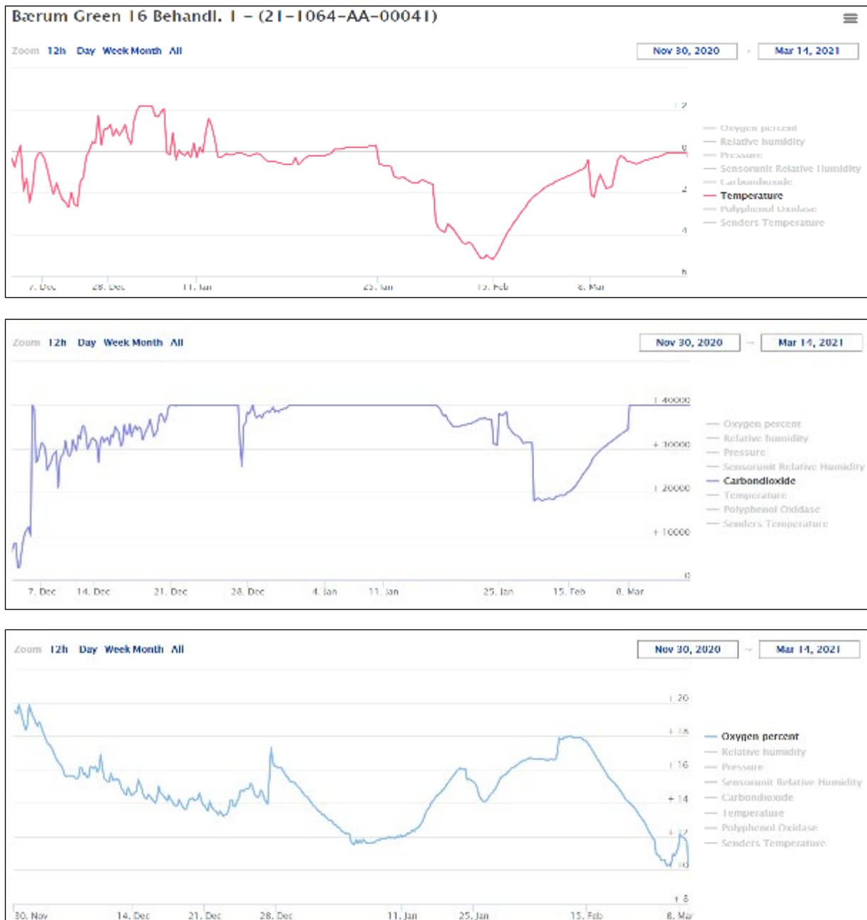
Figure 9a-c. Temperature and CO<sub>2</sub>- and O<sub>2</sub> concentrations under plastic sheets on the unventilated Green 16 at Bærum.
