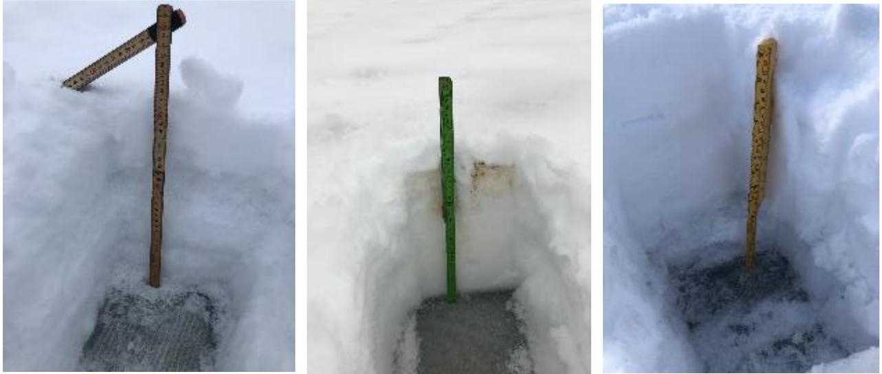
*Photo 14a-c. Snow depth and snow consistency at Bærum GC on a) 16 Feb., b) 22 Feb. og c) 12 March. A porous ice layer under the snow was not formed until a mild spell in mid February (b) The maximum ice + snow depth of about 40 cm was observed shortly before snow removal in mid-March. Photos: Guttorm Ray Tuxen.*
