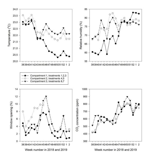
958 Figure 3: Weekly averages for temperature (oC), relative air humidity (%), ventilation opening (%)
