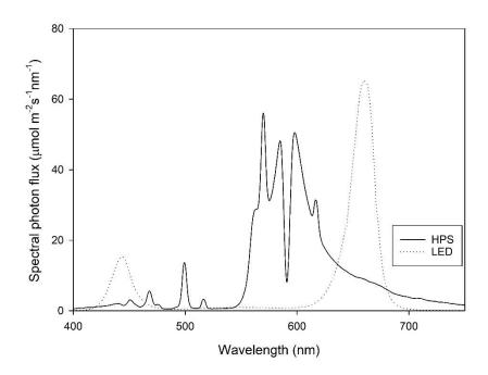
Figure 1. Spectral distributions of High Pressure Sodium (HPS) and Light Emitting Diode (LED) lampsused in the experiment.
