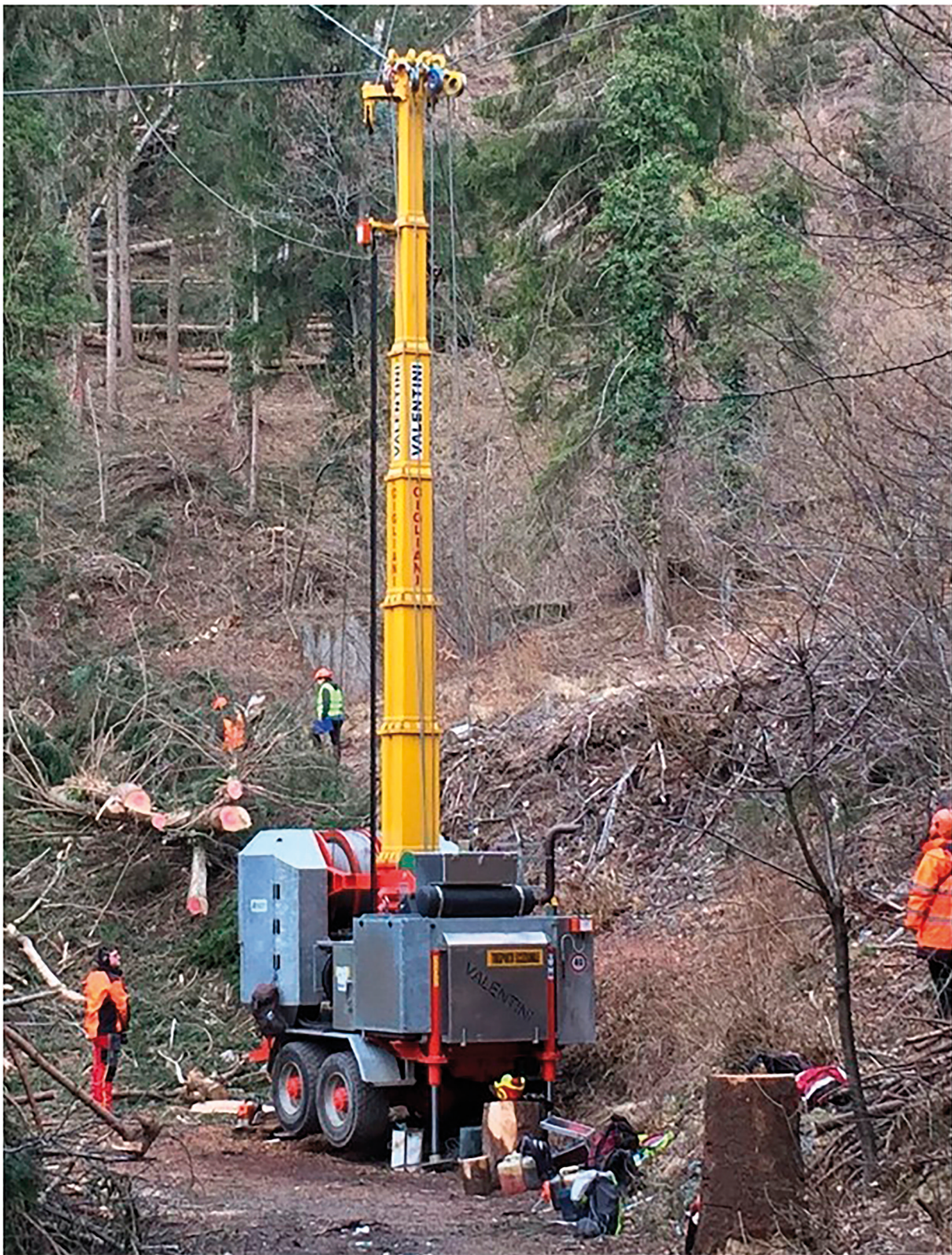
Figure 2. Valentini V850 M3 trailer-mounted tower model used to perform the study (photo credit: Giovanna Ottaviani Aalmo).
