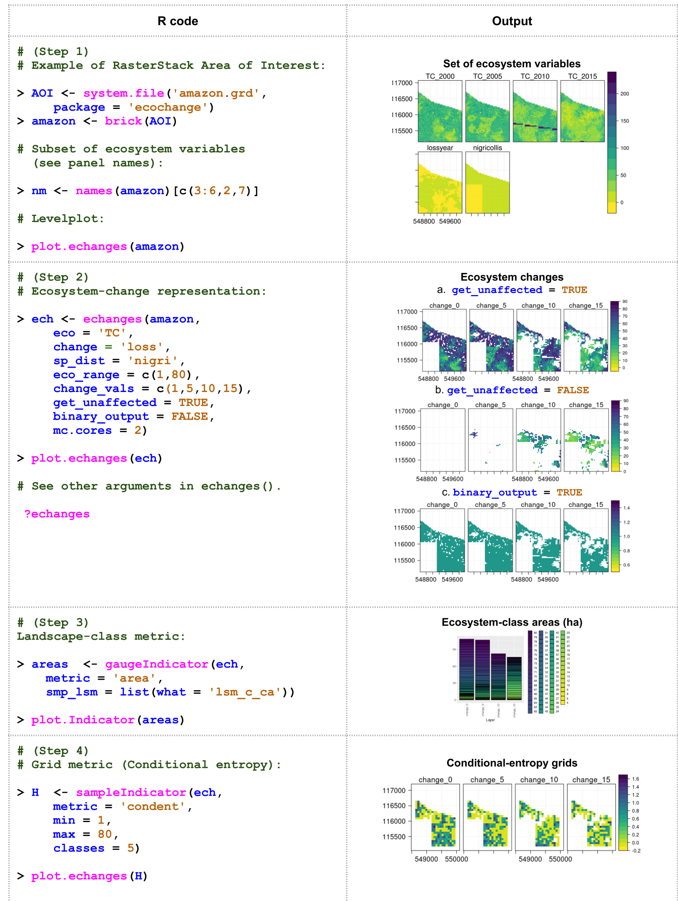
FIGURE 4 Example workflow to calculate ecosystem-class areas and conditional entropy processing a predefined RasterStack area of interest included in the package.
